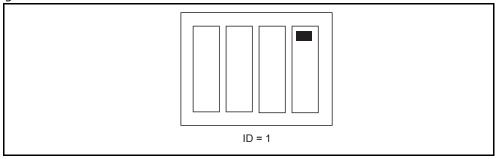
The LEDs will light (and remain steady) to indicate the address. For example, if the ID DIP Switch is set to 1, LEDS D1 will on. If the ID DIP Switch is set to 3, LEDS D1 and D2 will be on.
